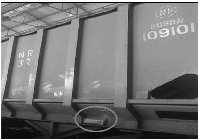
Figure 1 RFID tag fitted on a freight wagon in Indian Railways (pilot project).
